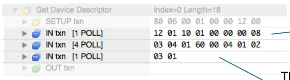
If the request has a non-zero length, the transfer has a data stage compromised of one or more IN or OUT data transactions.
