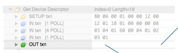
Each control transfer ends with a status stage, which confirms both sides agree that a transaction completed correctly.
