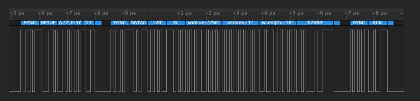
each control transfer is made up of a number of transactions...
